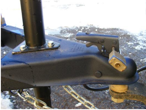
Hitch Coupler Secured on Ball.
