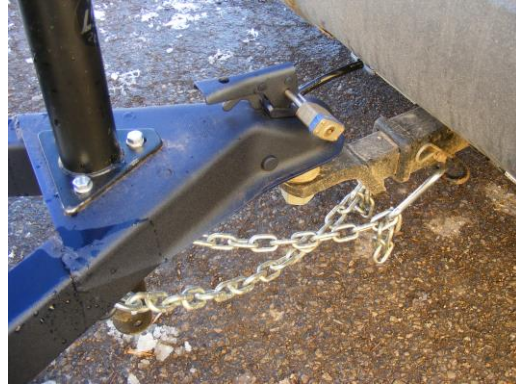
Correct Safety Chain Installation.
