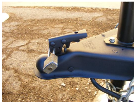
Hitch Latch Closed And Locked.
